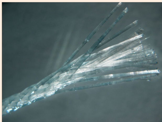
Figure 12: The resin impregnated in each fiber of each thread represents 6% of the mass and therefore its contraction after polymerization remains extremely slight and undetectable (less than 0.06%).
