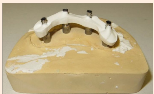
Figure 13-15: Spatial stability tests were carried out on a CST Link® type fiber-reinforced structure, coated with translucent silicone and polymerized on four posts, using a profile projector and doubled with 3D camera measurements: an average deviation of gap of 0.07% (between posts 1 and 3) were observed, which correspond to a gap of 19µm. Plaster control keys, built on a model replica, remained free of fractures and cracks, demonstrating the perfect passivity of the structures.
